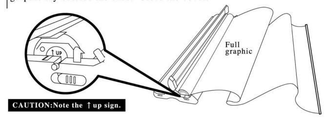
7. Push the graphic forward slightly to activate the spring system. Remove the locking pin and let the graphic retracts into the system slowly.
