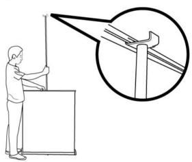
4. Pull up the second graphic and position the end tip of the pole into the profile.
