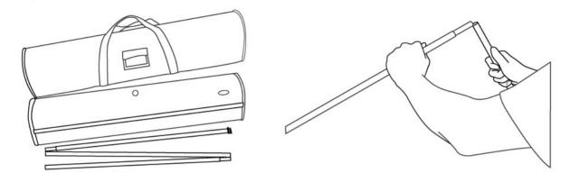
2. Insert the pole onto the cup of the base.
