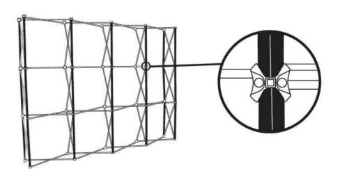
4. Attach the graphic hanger onto the top hub and adjust the position with the flexbility from the floating magnet.
