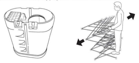
2. Once the frame is fully expanded, the magnetic arms will gently locks into place. If the magnetic arms are not locked together, then, the frame has not fully expanded yet.
