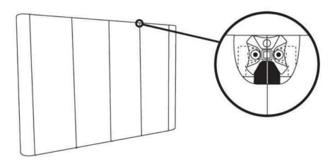
6. Gently slide the bottom of flood lights onto the frame top joints. The light will secure itself at the joint of scissors.
