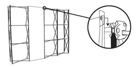
5. The graphic is secured with the magnetic hangers and channel bars.
